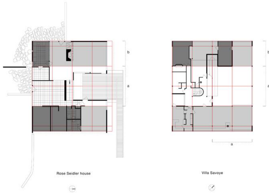
1. Proportional comparison of Villa Savoye and Rose Seidler House plans. [Drawing by I-wen Kuo]
