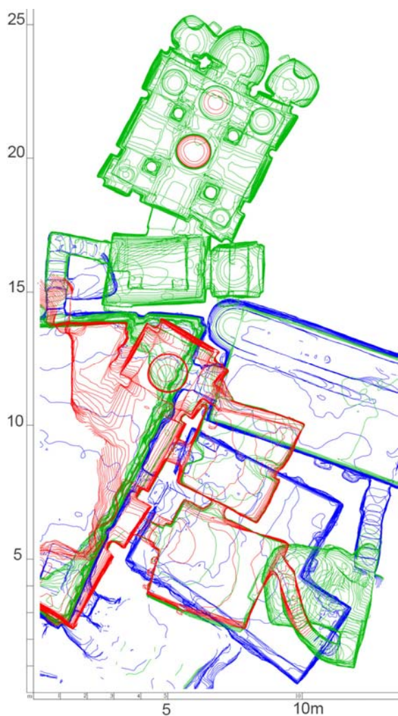
Figure 2: General plan, detail: lower level in blue; middle level in green; upper level in red. Karanlik Monastery
